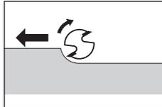
If milling proceeds in the direction of the router rotation (climb technique), the machine might be ripped out of the operator's hands.
