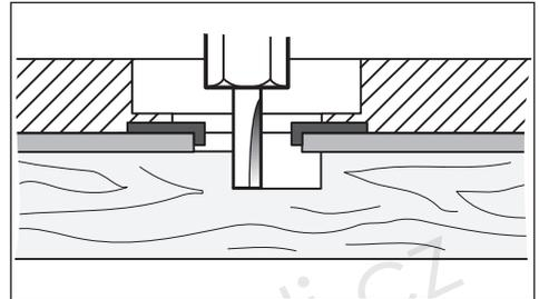
Press the clamping lever (8) and push the machine slowly down to the workpiece, until the adjusted milling depth is achieved.
