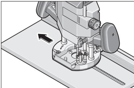
Lead the rear straight flat side of the skide (15) alongside the skid plate.
