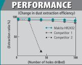
Built-in dust collection system with large dust bag and more surface area is 3x more efficient
